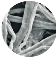
Cellulose Fiber at x500 Magnification
